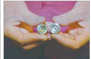
Parts with heavy oil loading before and after cleaning in an automated ultrasonic parts cleaning line.
