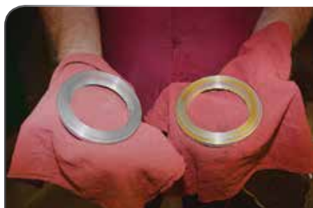
Heavy oil loading on "before" part is successfully removed on "after" part by ultrasonic cleaning.
