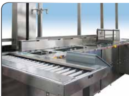
Multiple-station ultrasonic parts-cleaning line with conveyorized load and unload.
