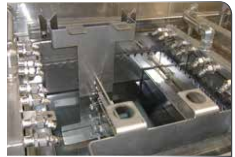
Ultrasonic cleaning tank with four-sided overflow weir and spray headers.
